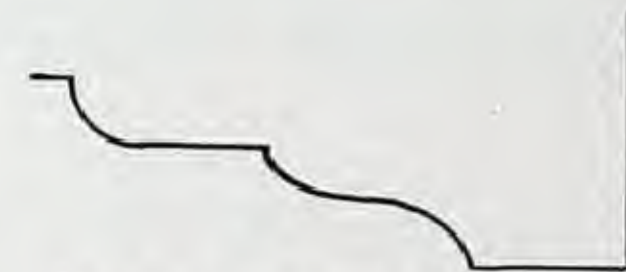
No. 934.—Angle moulding ; any size to suit.
